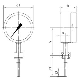
The sensitive portion I2 shall reach the media temperature completely. The insertion length I1 should have adaquate size.
