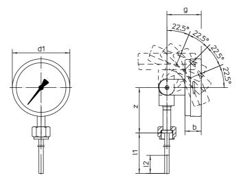
The sensitive portion I2 shall reach the media temperature completely. The insertion length I1 should have adaquate size.
