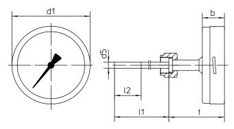
The sensitive portion I2 shall reach the media temperature completely. The insertion length I1 should have adaquate size.
